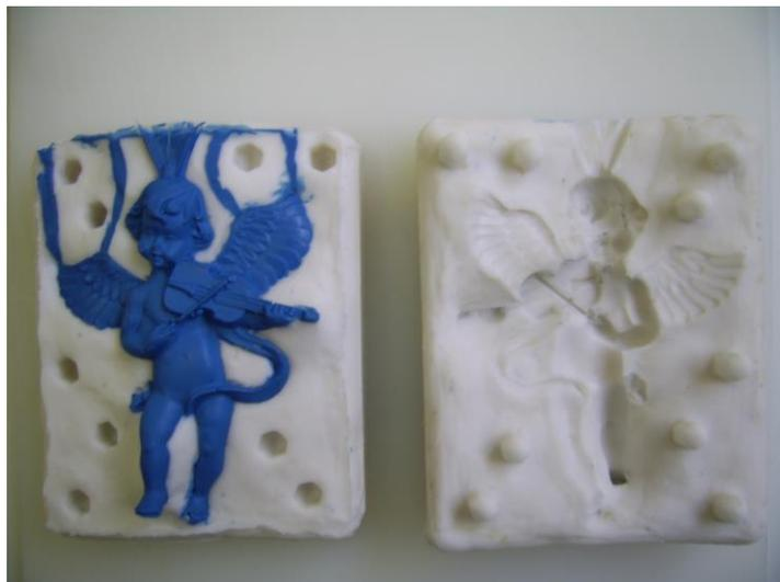
**28.** Reassemble the mould and try another casting. The cured casting when removed from the mould will have solid chimney pieces which will have to be trimmed off along with the pouring head.
