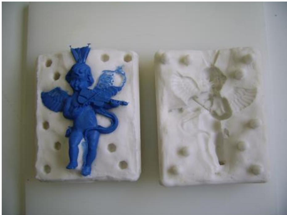
**27.** When there is a problem with air entrapment in certain areas, the problem can be remedied by using a sharp blade to scribe out very small V channels around 1mm deep on one half of the mould. The channels are cut from the air entrapment point right up to the top of the mould block creating “chimney” passages for air to escape. During the next casting a small amount of casting material should appear at the top of these chimneys.
