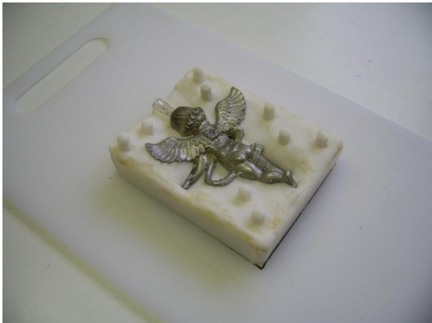
**17.** Place the silicone rubber back on the base board in the marked area and repeat steps 2 and 9. Next, to prevent the second pour of silicone rubber sticking to the cured block, brush a thin layer of warmed Vaseline over the silicone rubber around the exposed pattern half, avoid getting the Vaseline on the pattern as this will reduce the detail
