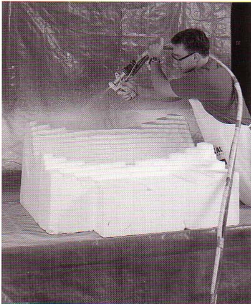
Spray RAYITE 200 on undersized armature.
