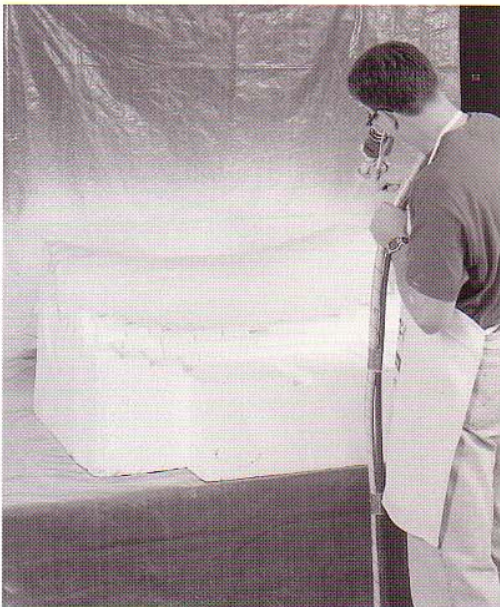
Spray RAYITE 200 to slightly oversized tolerance.
