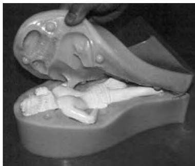
Poly 74-20 offers the most remarkable combination of tear strength and softness. With tear strength similar to harder rubbers, Poly 74-20 pulls away from detail and undercuts with no trouble at all. Poly 74-20 is great for casting concrete, plaster wax and resins.
