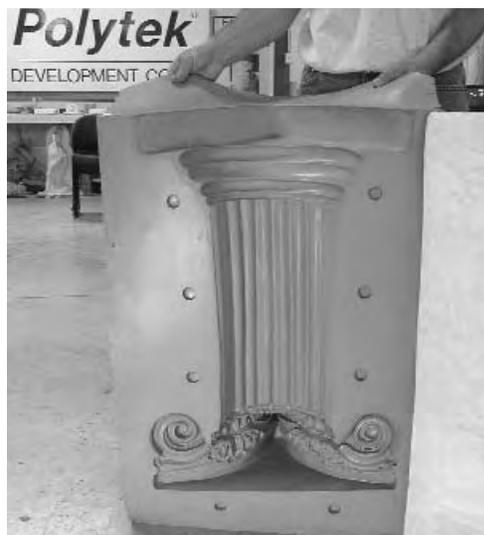
*This Polygel® mold was used to rotocast hollow plaster columns used routinely for home and office decor.*
