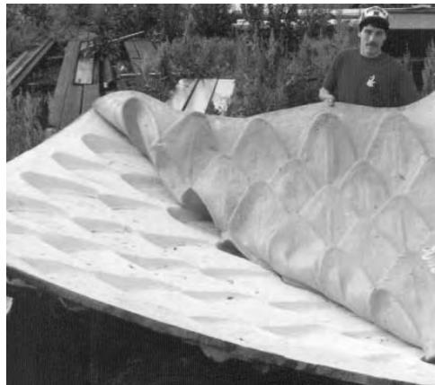
*A large, flexible rubber dome mold was made quickly using Polygel® Spray 50 for the restoration of the St. Joseph County Courthouse in Southbend, IN.*
