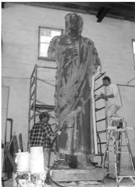
*Polygel® Spray 50 is applied to a monumental sculpture with the VS-3000 Polygel Sprayer (see p. 64). Using the sprayer, the entire mold was made in a continuous sprayed piece. The gel emitting from the sprayer is non-sag and, therefore, stays where it is applied, but can be moved around with a brush if necessary.*
