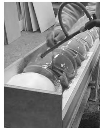
*Polygel® Mold Rubbers are specifically designed for brush-on and spray application. After Parts A+B are mixed, they form a thixotropic gel that clings to vertical and overhang surfaces after application.*
