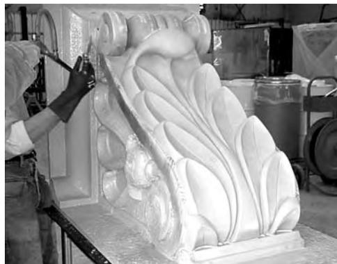
*Using Polygel® Spray 50 a mold was made of this this large cornice bracket.*
