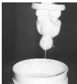
Latex False Face molds can be made by dipping a dry, porous plaster model into False Face. The longer the model is submerged, the thicker the mold. This technique is only suitable for models with a shape that won't trap air when placed upside down in the False Face liquid.
